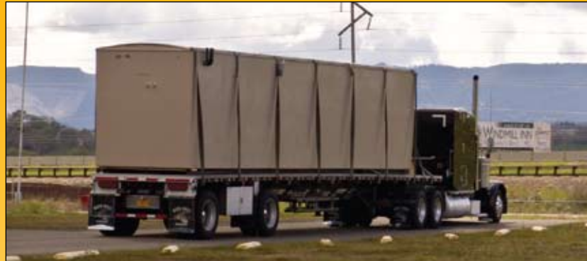
▲ The largest AX-Mobile™ unit weighs 10,000 lbs (4,536 kg), and can be transported by truck, rail, cargo container, or helicopter.
